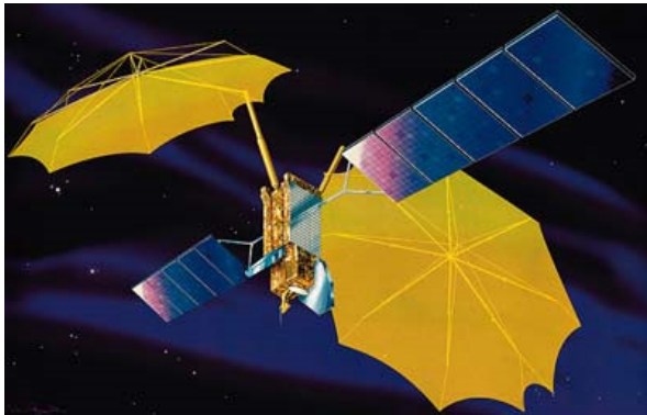
Fig. 5. Garuda-1 (ACeS-1) design, two times 12 m antenna diameter (Lockheed-Martin via Gunter's Space Page)
