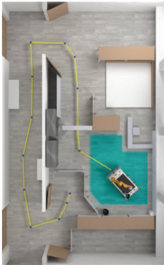
FIGURE 23: Kidnapped robot problem: a robot is randomly placed in a predefined area (green) in a known map. After self-localization the robot plans a path (yellow) to its goal.
