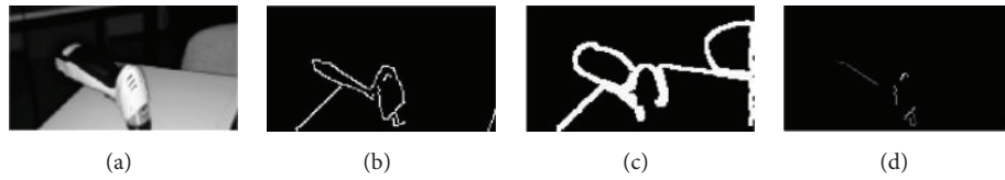
FIGURE 6: Edges detected in cropped ToF data. From (a) to (d) intensity, intensity edges, range edges, and edge difference image. In the intensity image the color gradient of the handle of the power screwdriver being used as a feature is conspicuous. This gradient can be recognized in the (d) difference image again.
