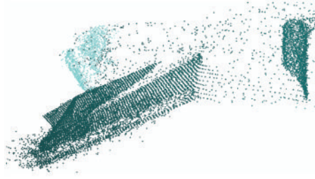
FIGURE 4: The noise in a ToF cam depth image prevents reliable geometric feature calculation. The power screwdriver is colored light blue.
