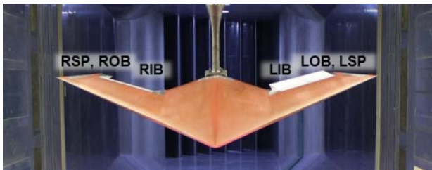
Fig. 3 DLR-F19 in the DNW-NWB closed test section (mounted top down on a belly sting). LIB/LOB label the left inboard/outboard control surfaces and RIB/ROB the right inboard/outboard control surfaces, respectively. RSP/LSP stands for right and left split flaps.
