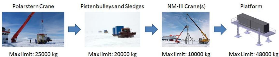
**Figure 5. The rough mass limits of the Neumayer Station III logistics chain as an example for Antarctic greenhouse shipment considerations.**
