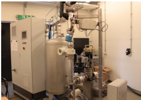
Figure 4.54: Test facility for heat exchanger. Fore-ground: controller unit. Background: Water test bench consisting of a water circle circuit with heater, switch cabinet, water tank, centrifugal pump and to be tested evaporation cooler in the upper part of set up.
