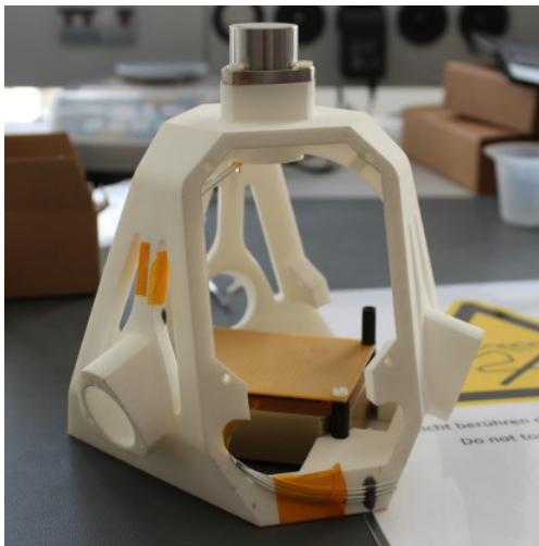
Figure 4.13: Laboratory prototype for the inertial measurement unit in redundant (tetraaxial) configuration developed for the ReFEx Hybrid Navigation System (HNS) .
