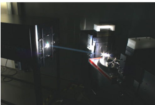
Figure 4.3: Sun sensor verification in the laboratory STARS using a Sun-equivalent light source and a rotation table to verify sensor accuracy and behaviour at high spin rates.
