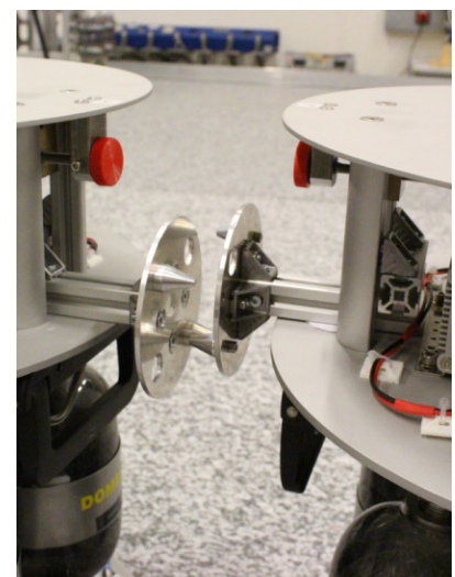
Figure 4.1: Two TEAMS vehicles are about to make a docking. Demonstration of model predictive control for rendezvous and docking with an uncooperative rotating target.
