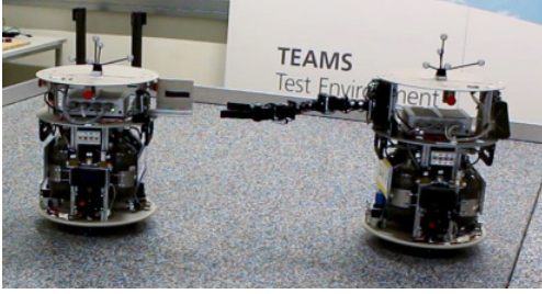
Figure 4.7: Two TEAMS vehicles simulating client and servicer spacecraft. Demonstration of GNC algorithms for capturing an uncooperative rotating target.
