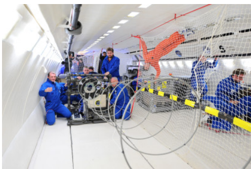
Figure 4.67: Deployment testing of the AlSat helical Antenna on the 15. Parabolic Flight Campaign of DLR 2010 in Bourdeaux.
