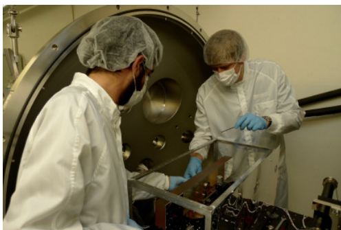
Figure 4.59: Scientists aligning the reference plate as part of the OGSE for verification of the GRACE-FO laser ranging instrument.
