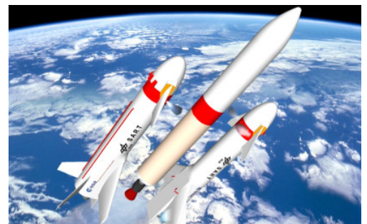
Figure 2.5: ASTRA Liquid Fly-Back Booster (LFBB) at staging from core stage in artist's impression.
