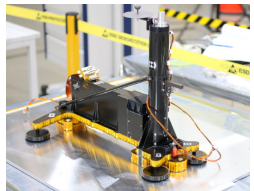
Figure 3.39: FM integration of support system assembly, i. e. the support system including the mole under planetary protection conditions.
