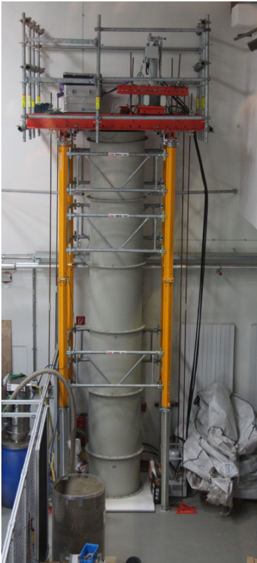
Figure 3.41: Deep penetration test bed used for mole development as well as for qualification tests (e. g. life test).
