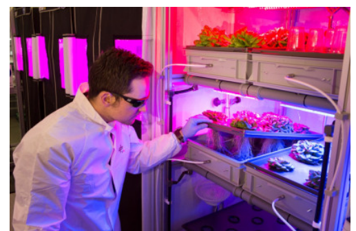
Figure 4.70: Multilevel plant growth systems within the EDEN laboratory employing aeroponics and water-cooled LED lighting.
