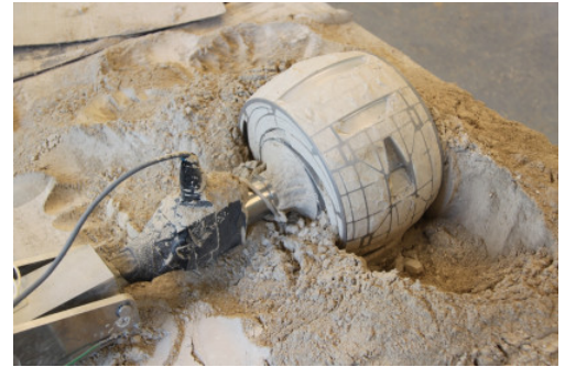
Figure 4.43: Mars Exploration Rover (MER) wheel in single wheel test bed, representing the situation of MER-A during 2009. Despite extended studies and laboratory test campaigns to optimize the driving and locomotion strategy, the rover could not be retrieved from the sandy terrain.
