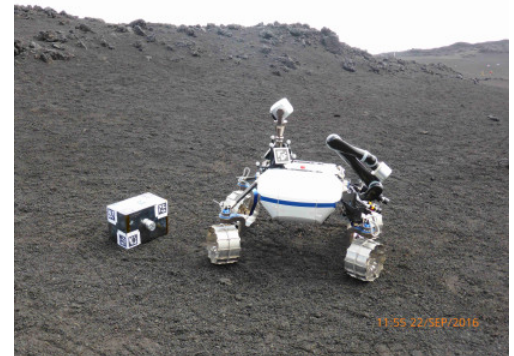
Figure 4.38: Remote unit (seismic station) after deployment by rover during pre-test at Mt. Etna.
