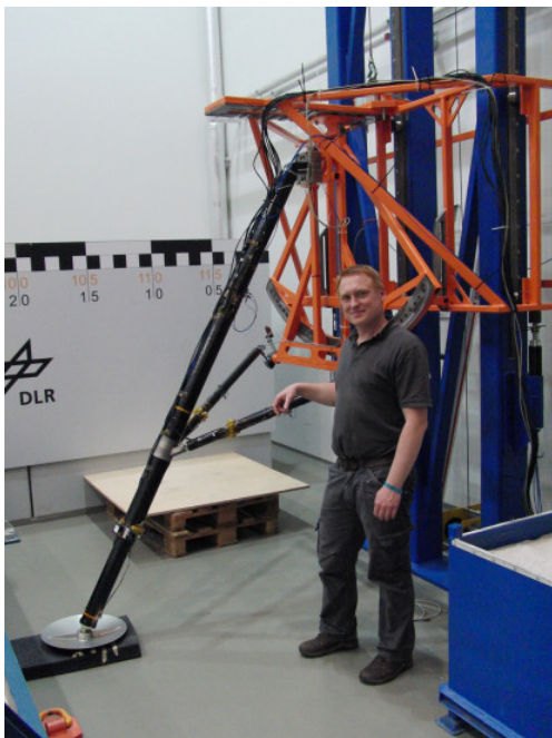
Figure 4.47: Single leg test stand with full-scale ESA Lunar Lander leg engineering model.
