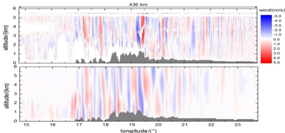
Figure 3. Top: Corrected vertical winds derived from lidar measurements performed on a research flight (13. December 2013). Bottom: Corresponding vertical wind speed from WRF-model.
