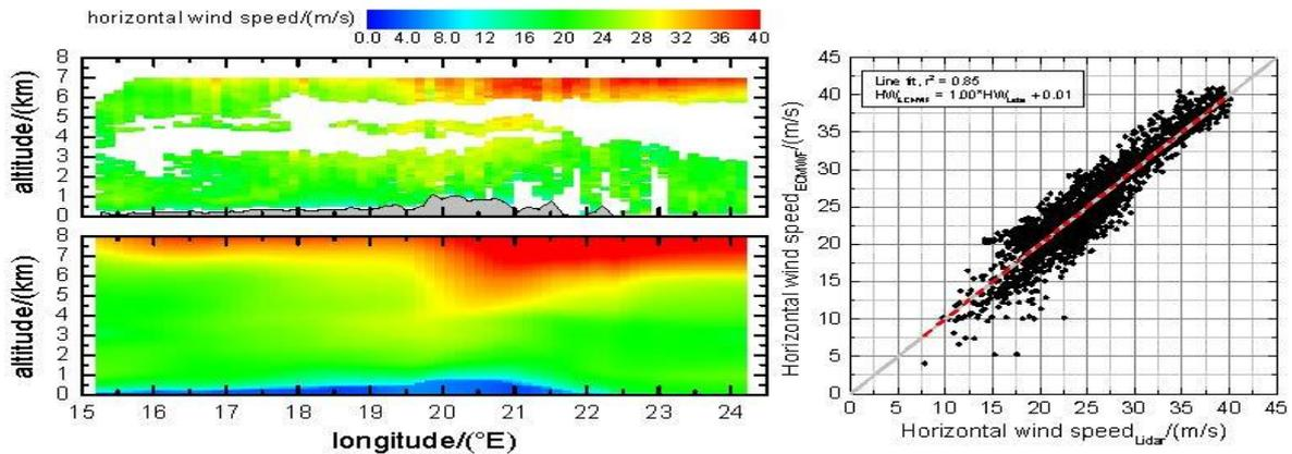
Figure 2. Left, top: Horizontal wind speed derived from lidar measurements. Left, bottom: Horizontal wind from ECMWF re-analysis data. Right: Lidar vs. ECMWF, line fit (red) and  $x=y$  line (gray).
