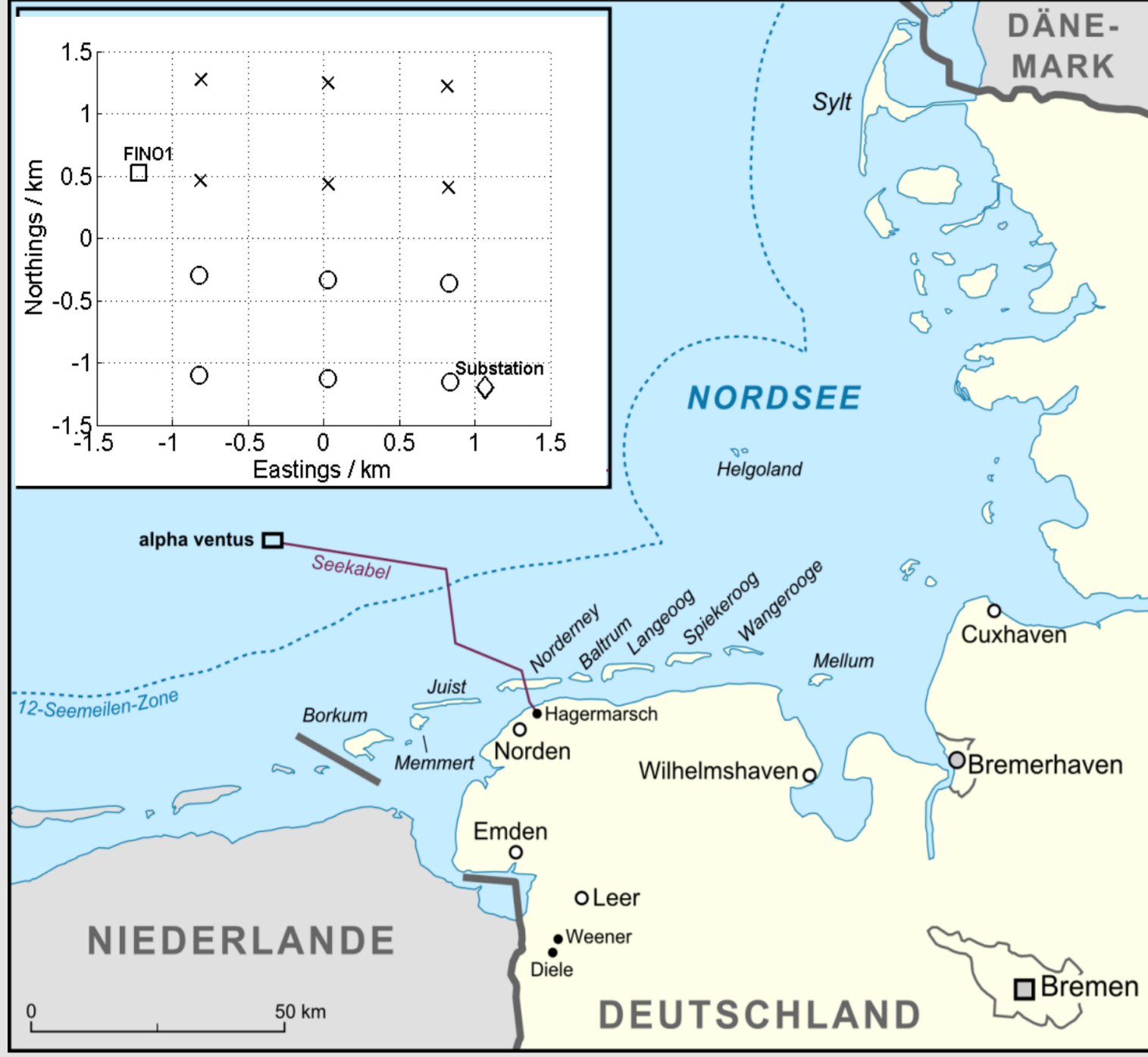
Figure 1. Location and layout of the offshore wind farm alpha ventus. Crosses and circles indicate different turbine types with diameters of 126 m and 116 m (two southerly rows). One LiDAR was operated on the substation (◊) and two on the research platform Fino1 (◻).
