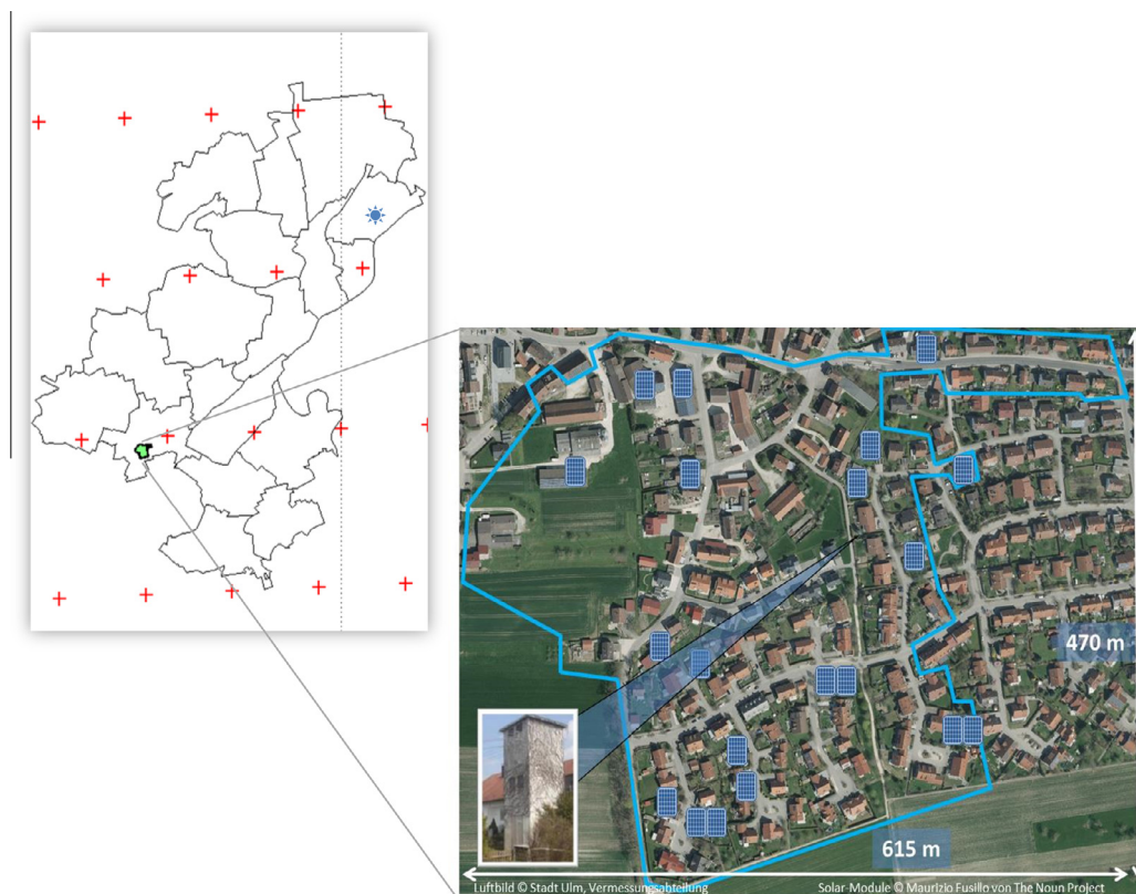
Fig. 3. Overview of the test site location (green-filled polygon), location of the ground-measured irradiance (blue star) and the pixel-size of the MSG satellite (pixel corners are marked with red crosses). Grey lines indicate the different districts of ULM. (For interpretation of the references to color in this figure legend, the reader is referred to the web version of this article.)
