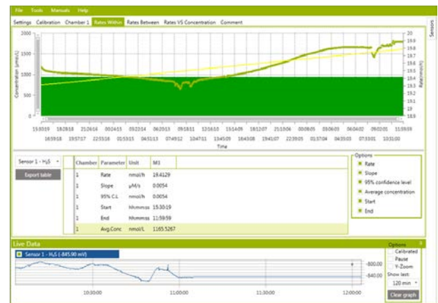
Fig. 1 Monitoring of a growing Desulfovibrio sp. culture for H 2 S production. pH changed during the growth from 7 to 5.9 after several days.
