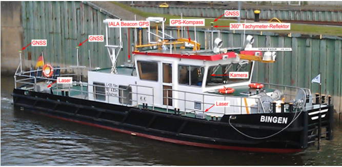
Fig. 2. Research vessel “MS Bingen” used in the measurement campaign and the corresponding measurement equipment
