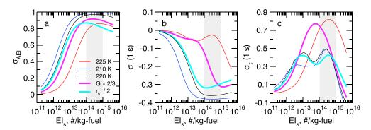
**Figure 3.** Dependence of contrail ice particle (a) number, (b) radius, and (c) optical depth on the soot number emission index. Conditions as in Figure 2.
