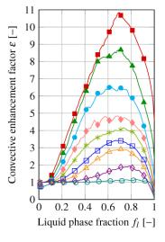
Figure 6: Convective enhancement factor over liquid phase fraction
