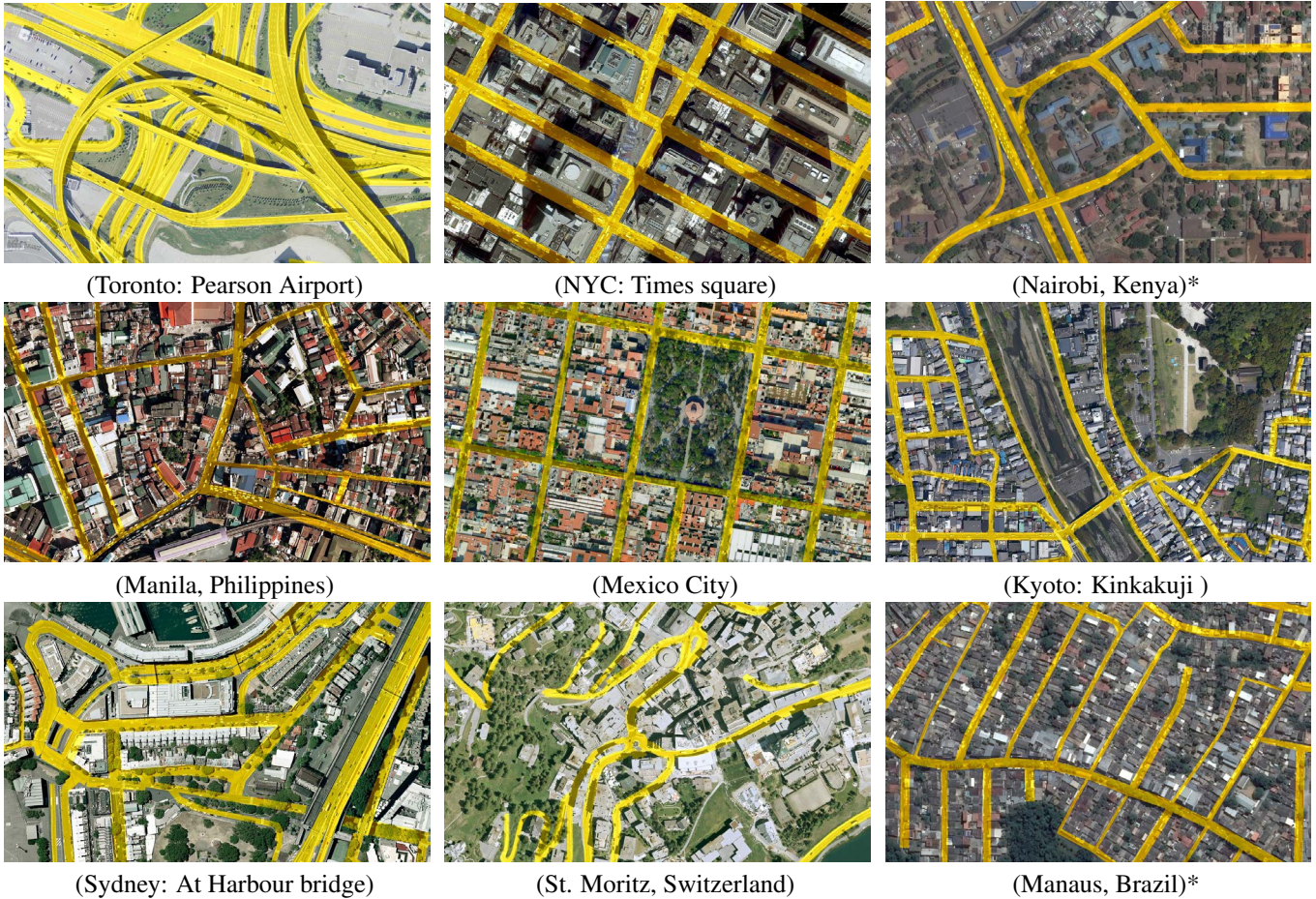
Figure 4. Segmentation results on several cities over the world using the edge, homogeneity, context, car and overlap features. Note that the MRF was trained only on 1.5 \text{ km}^2 imagery from the Aerial KITTI dataset. * Indicates satellite image.
