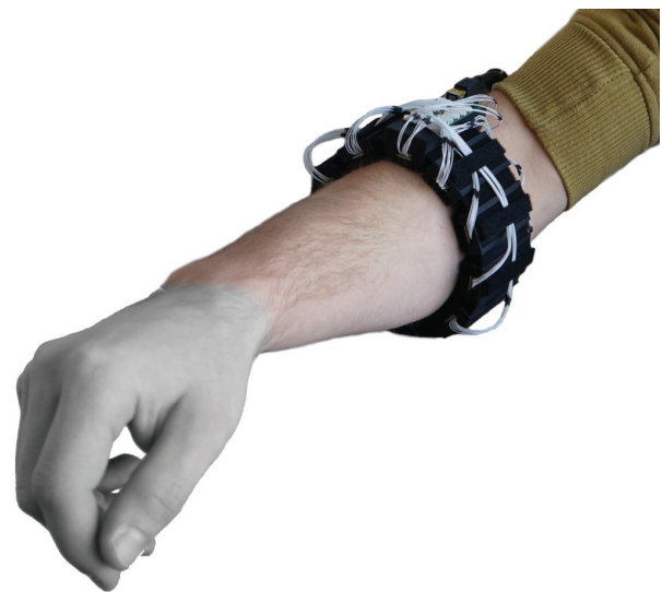
Fig. 1. A high-spatial resolution tactile bracelet with a soft and conformable shape is used to capture muscle activity in the lower forearm. One possible usage scenario for this bracelet would be to capture hand amputee intention in order to drive the single fingers of a modern multi-DOF hand prostheses.
